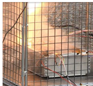
Figure 13. Test Battery induced into thermal runaway
