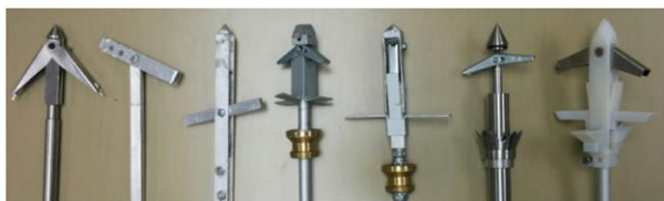
Figure 9. Harpoon projectile prototypes and evolution.
