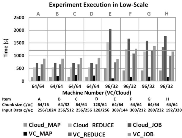
Fig. 3. Low Scale - 128 Machines - 10 Mbps - Tasks > Resources
