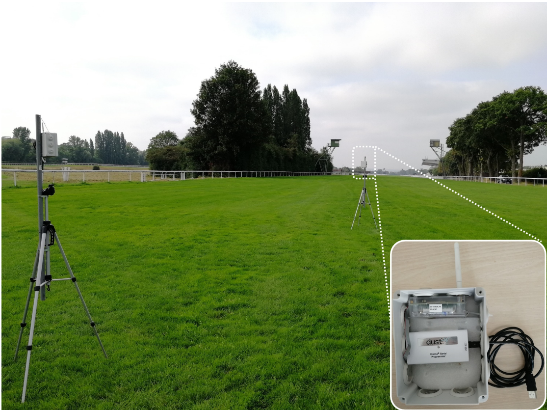
Figure 3: A box contains a mote and a DC9010, used to interface the mote to a computer.
