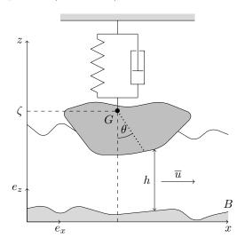
FIGURE 7. Wave energy converter with a spring
