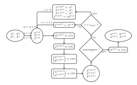
FIGURE 2. Scheme of the weak coupling iterative process. The notation  $a \leftarrow b$  is the numerical affectation, i.e. a gets the value of b. The notation  $a \Leftarrow (X)$  means that a is computed using the equation (X).
