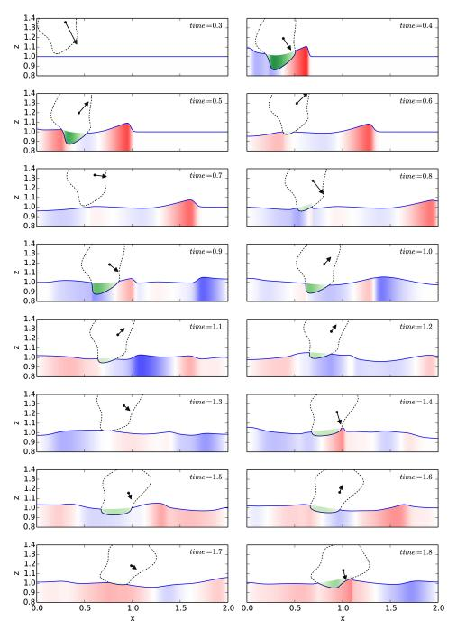
FIGURE 5. Throwing: Buoy (black dotted line), water height (blue solid line), velocity (filled surface in the water – blue < 0 < red) and surface pressure (green filled surface in the buoy) at several times.
