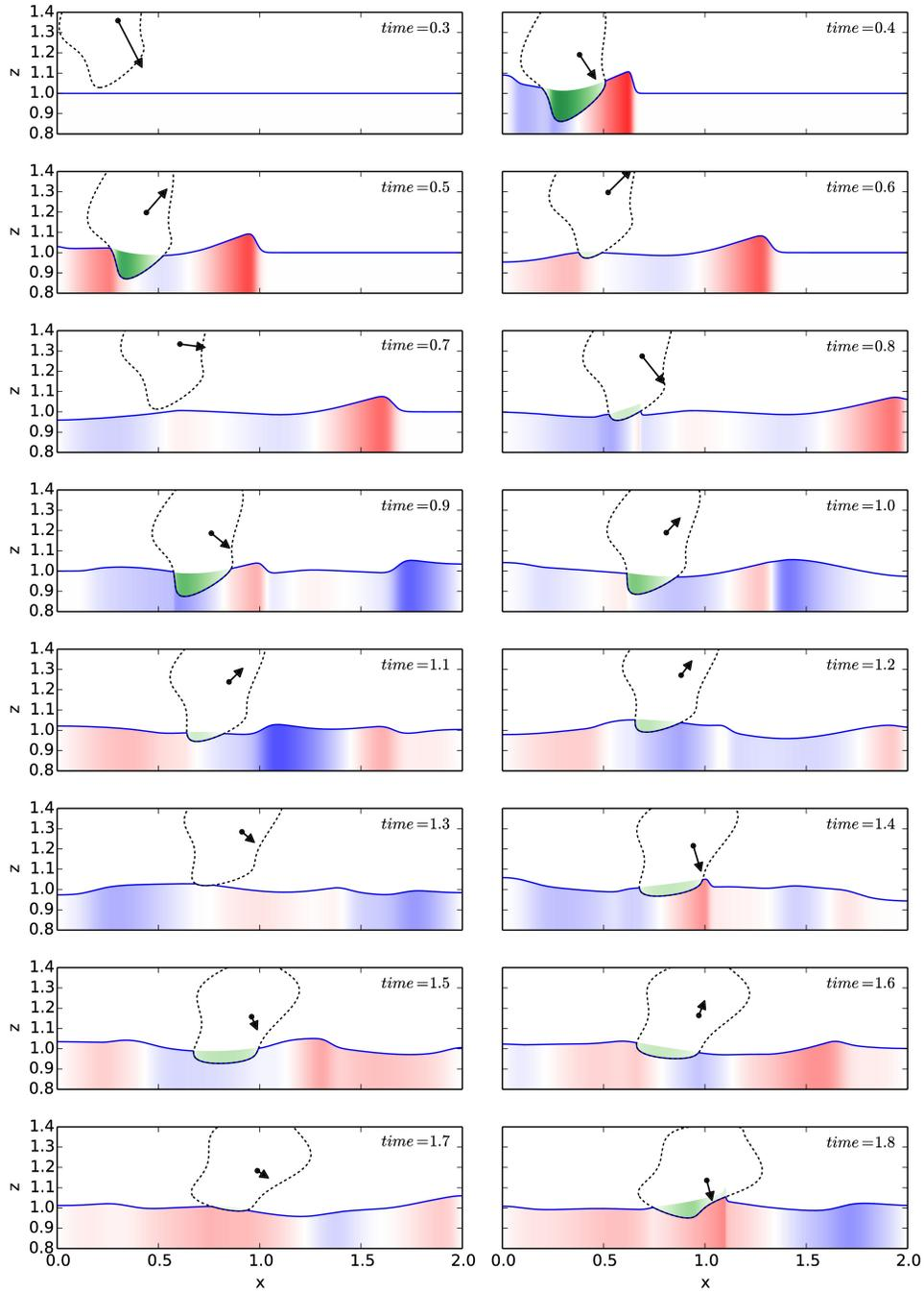
FIGURE 5. Throwing: Buoy (black dotted line), water height (blue solid line), velocity (filled surface in the water – blue  $<0$   $>$  red) and surface pressure (green filled surface in the buoy) at several times.
