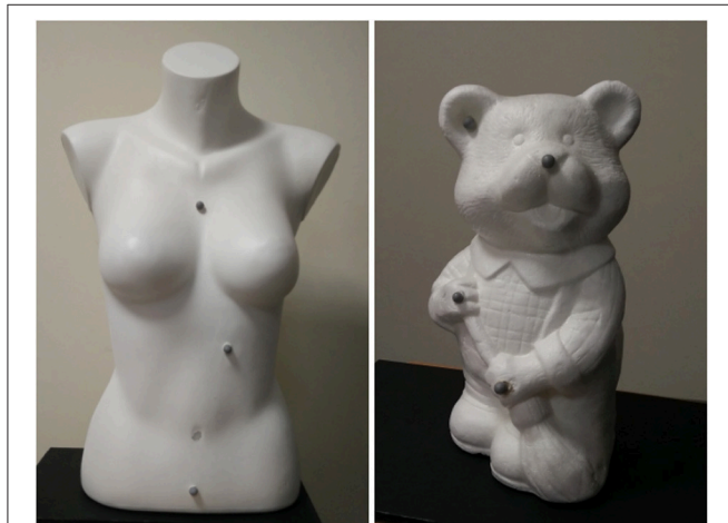
FIGURE 4 | Examples of tangible objects augmented with MoSART. The objects are white or covered with white painting. Reflective markers are positioned over the objects to facilitate their localization.
