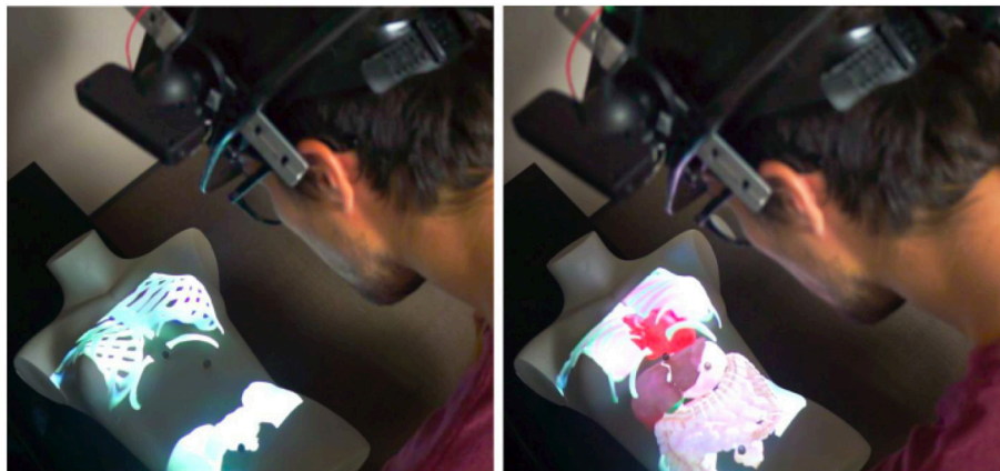
FIGURE 12 | Medical visualization on a tangible chest. The user is able to visualize the bones ( Left ) with or without the organs ( Right ). [This image is published with the written and informed consent of the depicted individual(s)].
