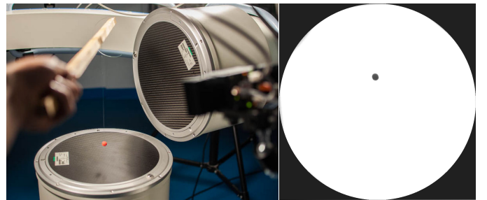
Fig. 6. Calibration ball. Left: cropped video input from a selected camera; right: radiographic image. While 2 C-arms are visible in this image, a single one is used in this work.
