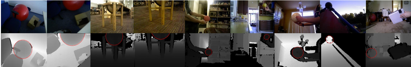
Figure 7. Qualitative visualizations of sphere detection in the wild: Our algorithm is very successful in difficult scenarios including clutter, occlusions, large distances. Note that the sphere is detected in 3D only using the point clouds of depth images and we draw the apparent contour of the quadric. The RGB pictures are also included in the top row to ease the visual perception.
