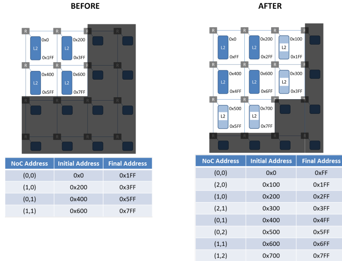
Fig. 3. ATA table and MPSoC before and after resource distribution.
