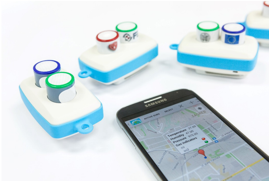
Figure 3. Wearable sensors for air quality monitoring 2
