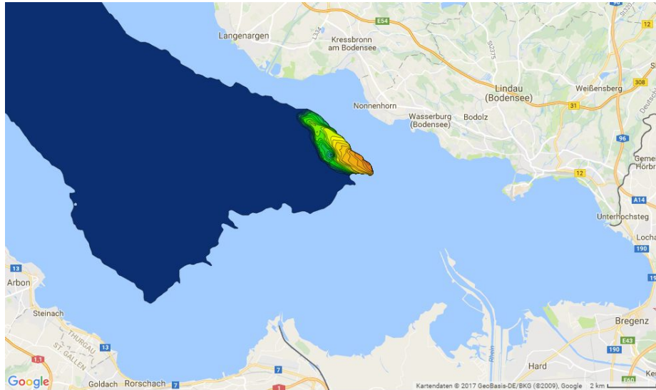
Fig. 1. 2D slice at 140m water depth visualizing suspended sediment concentration
