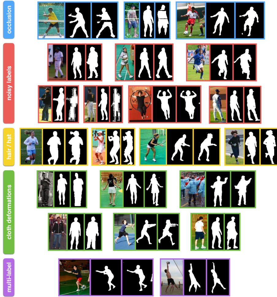
Fig. A.1: Projected silhouettes of our voxel predictions (middle) versus manually annotated segmentations (right) on the Unite the People dataset. We note that the evaluation is problematic due to several reasons such as occlusions and clothings, whose definitions are application-dependent, i.e., one might be interested in anatomic body or the full cloth deformation.
