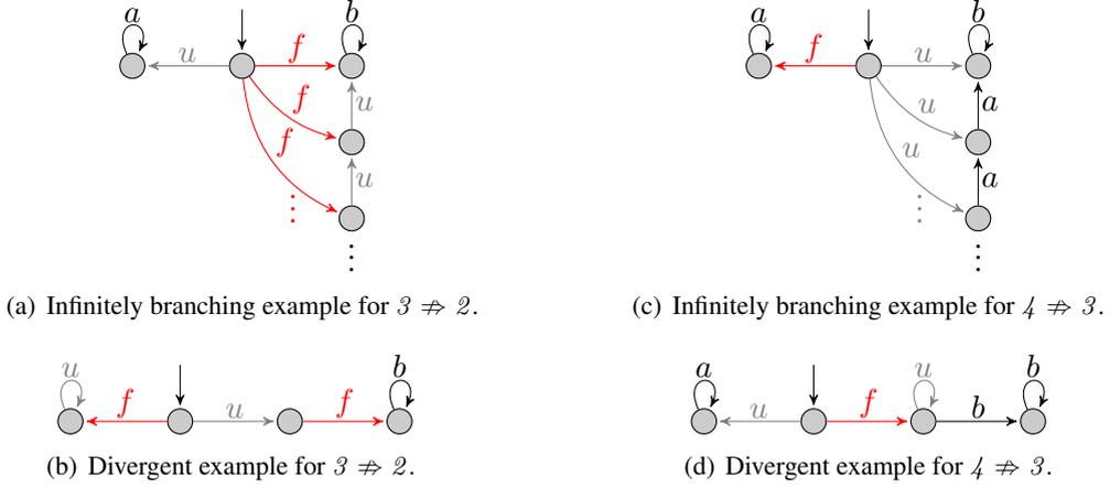
Figure 6. Counter-examples for Lemma 2.6, with  $\mathcal{O}(u) = \mathcal{O}(f) = \varepsilon$ ,  $\mathcal{O}(a) = a$ , and  $\mathcal{O}(b) = b$ . The LTSs on the left are finitely diagnosable but not dynamically diagnosable while those on the right are trace-diagnosable but not finitely diagnosable.
