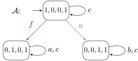
Figure 1. Example of a partially observable system.
