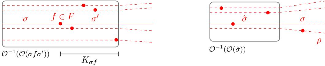
(a) Illustration of dynamic diagnosability. Each line represents a trace in  $\mathcal{A}$  whose observation starts with  $\mathcal{O}(\sigma f \sigma')$ , and bullets indicate faults. Each trace must contain a fault at most  $K_{\sigma f}$  steps after the earliest possible fault occurrence.
