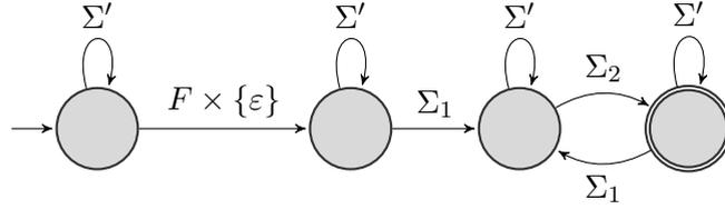
Figure 4. A Büchi automaton  $\mathcal{B}_{\text{diag}}$  for trace-diagnosability.
