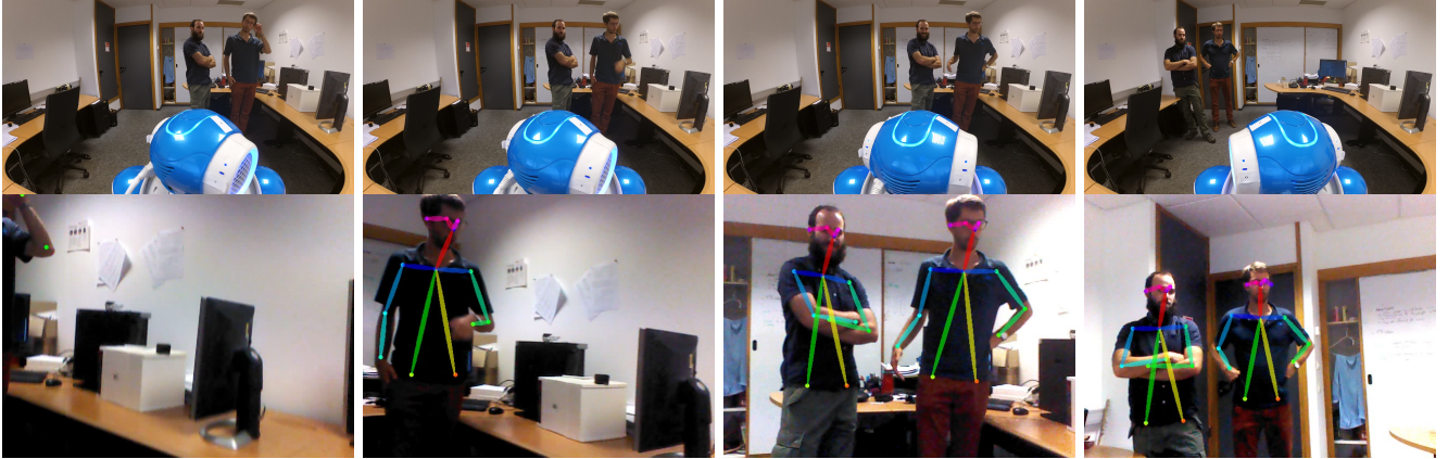
Fig. 5: Example of a live sequence with two persons. First row shows an overview of the scene, including the participants and the robot. Second row shows the images gathered with the camera mounted onto the robot head. The robot head is first initialized in a position where no face is visible (first column), and the model uses the available landmarks (elbow and wrist) to find the person onto the right (second column). The robot detects the second person by looking around while keeping the first person in its field of view (third column), and gazes the two people walking together (fourth column).
