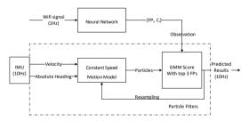
Fig. 3. Fusion of IMU and WiFi using GMM Particle Filter
