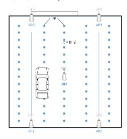
Fig. 1. Illustration of offline phases in WiFi Fingerprinting
