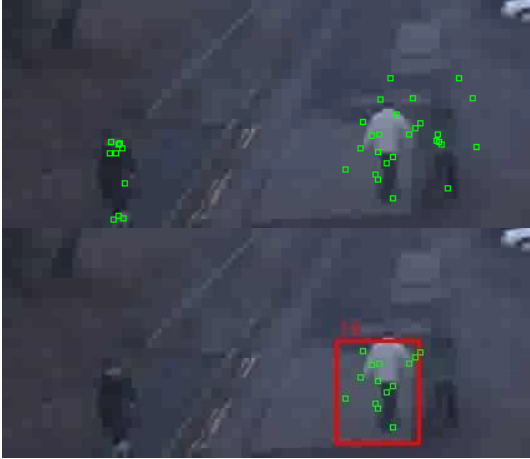
Fig. 6. Dense tracklets extracted (top): from the whole frame includes the motion from all moving objects in the scene, (bottom): from the bounding box of the tracked object that contains only the motion related to the object of interest.
