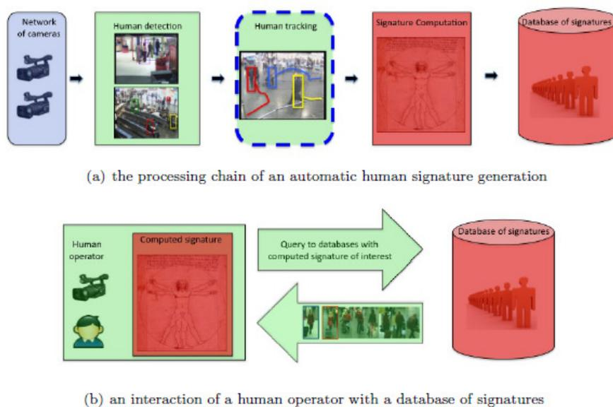
**Fig. 2** Overview of the proposed Re-ID process
