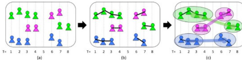
**Fig. 5** General Overview of the tracking approach in  $T$  frames: (a) The raw detection results; (b) the tracking results; (c) the results of matching trajectories using online discriminative appearances
