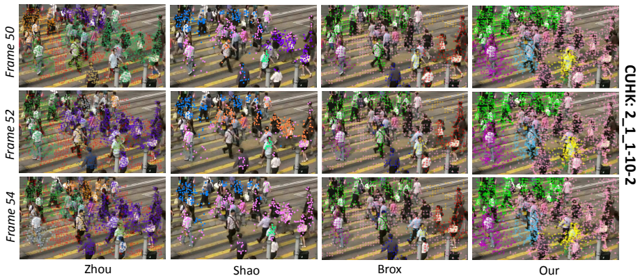
Fig. 1. Segmented motion patterns (or groups segregation) as the crowd evolves in time. The color of point represents the assignment to a group. While groupings are temporally consistent over a set of frames for Brox [2] and Our method. Zhou [3] and Shao [4] fail to maintain consistent groupings between frames.
