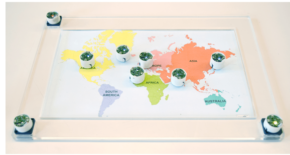
Fig. 7. By placing Latitude and Longitude magnets in the sandbox, the scatterplot become a map, showing the city of origin of applicants.
