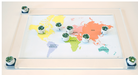
Fig. 7. By placing Latitude and Longitude magnets in the sandbox, the scatterplot become a map, showing the city of origin of applicants.
