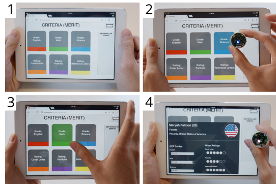
Fig. 4. Tablet interface to the applicant dataset: 1) The main attributes of the dataset; 2) A magnet is created by placing and holding a Zooid on an attribute; 3) Touching an attribute visualizes the values on each Zooid, through LED brightness; 4) Details are displayed on an applicant when their Zooid is placed in a dedicated area.
