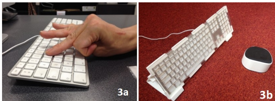
Figure 3a: YN's particular hand position while typing that sometimes causes accidental key presses and made the use of a keyguard slightly uncomfortable. Figure 3b: the DIY keyguard on its stands and the mobile armrest.
