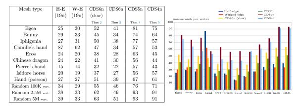
Table 3: Vertex degree computation: this table reports the average runtimes of our compact data structures compared to array-based implementations of the *Half-edge* and *Winged-edge* data structures (all results are expressed in nanoseconds per vertex).
