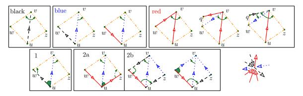
Figure 4: More compact scheme. Neighboring relations between edges are represented by tiny oriented (green) arcs corresponding to stored references, and by filled (green) corners that implicitly describe adjacency relations between outgoing edges incident to the same vertex: because of local Schnyder rule, we do not need to store references between neighboring outgoing edges.
