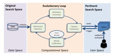
**Fig. 1** The Evolutionary Visual Exploration Framework (EVE). Raw data dimensions (from the data space) are fed into an evolutionary loop in order to progressively evolve new interesting views to the user. The criteria for deciding on the pertinence of the new views is specified through a combination of automatically calculated metrics (from the computational space) and user interactions (at the user space).
