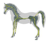
Figure 3: **Medial axis** (dark gray) and a **curve skeleton** (yellow) of a 3D shape. The medial axis is obtained using [35] and curve skeleton using [32]. This curve skeleton preserves the topology of the shape (light gray) and captures its features (ears, head, legs, tail).
