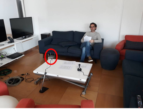
Fig. 8. Layout of the living room for the real recordings. The Eigenmike used for the recordings is circled in red.
