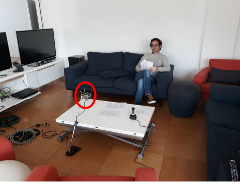
Fig. 9. Layout of the living room for the real recordings. The Eigenmike used for the recordings is circled in red.
