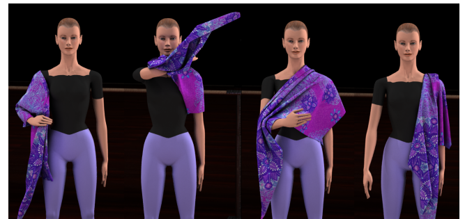
Fig. 13. Shawl demo, with \mu = 0.6 . The character grasps the shawl thanks to contact and Coulomb friction, and then throws it around her left shoulder. Finally the shawl slightly rolls over the shoulder due to gravity and friction. With a lower friction coefficient, the character is unable to grasp the shawl as it is too slippery.
