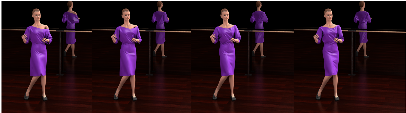
Fig. 1. Our implicit solver simultaneously resolves cloth elasticity, non-penetration and exact Coulomb friction constraints at every body-cloth and cloth-cloth contact, largely improving physical realism over previous methods. This new solver especially allows us to simulate accurately the effect of a varying friction coefficient \mu , capturing a diversity of cloth sliding motions and folding patterns as shown in this batwing dress example (from left to right, \mu = 0 , \mu = 0.1 , \mu = 0.3 , and \mu = 0.6 ). In this example featuring 2,600 contact points on average, our solver converges at each time step ( dt = 2ms ) to a high precision in a few hundred milliseconds only.
