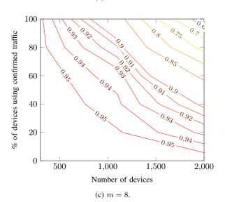
Fig. 2: Packet success rate for different values of m.
