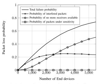
Fig. 3: Causes of packet losses with confirmed traffic.
