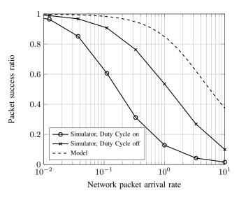
Fig. 5: Comparison of lorawan simulator with analytical model taken from [4].
