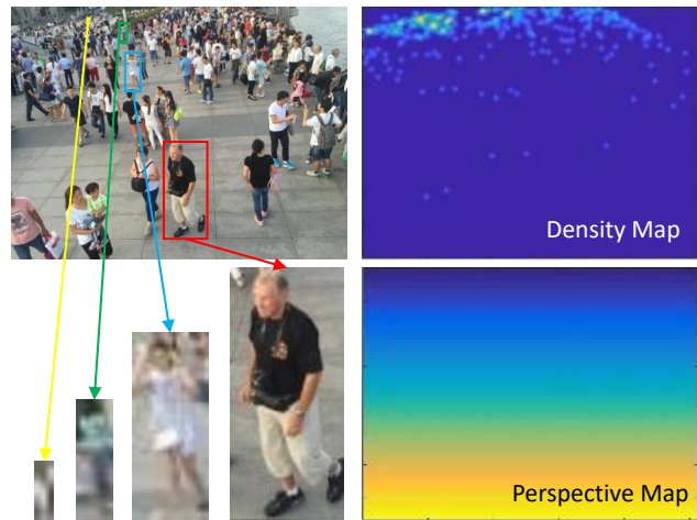
Figure 1: The density map shows the locally smoothed crowd count at every location in the image. The perspective map reflects the perspective distortion at every location in the image, e.g. how many pixels correspond to a human height of one meter at each location [46]. Person scale changes drastically due to the perspective distortion. Density regression on the small person area is in general very hard. We integrate the perspective map into density regression to provide additional information about the general person scale change from near to far in the image.
