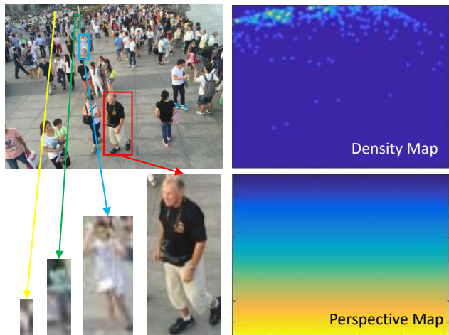
Figure 1: The density map shows the locally smoothed crowd count at every location in the image. The perspective map reflects the perspective distortion at every location in the image, e.g. how many pixels correspond to a human height of one meter at each location [45]. Person scale changes drastically due to the perspective distortion. Density regression on the small person area is in general very hard. We integrate the perspective map into density regression to provide additional information about the general person scale change from near to far in the image.
