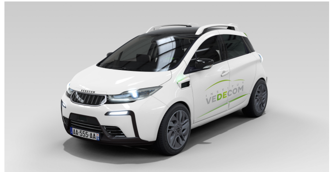
Fig. 4. VEDECOM Institute experimental platform. The car is equipped with 5 IBEO-Lux laser scanners with a high resolution IMU fused with an RTK-GPS receiver.
