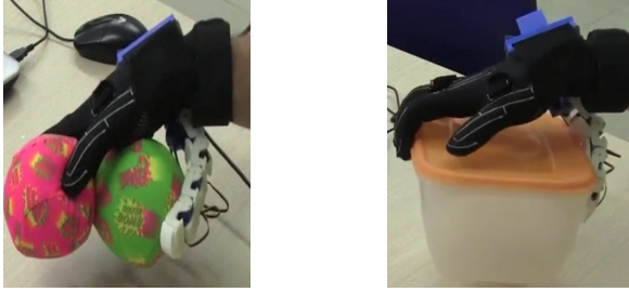
Figure 1.11: Fully actuated extra finger to enhance the capabilities of a healthy human hand. Left: grasping multiple objects in one augmented hand (ulnar grasp). Right: grasp of a big object (anatomically impossible grasp).
