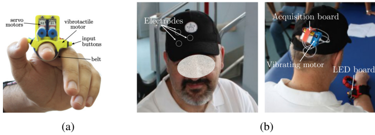
Figure 1.12: Possible interfaces for supernumerary limbs. (a) The hRing: It consists of two servo motors, a vibrotactile motor, two pairs of push buttons, and a belt. (b) The frontalis muscle cap: It is an EMG interface where electrodes are placed inside the cap at front side to be positioned on the patients forehead. The acquisition board and a vibrating motor are placed in a box on the back of the cap. An LED board at the base of robotic finger shows the activation of trigger signal and status of device.
