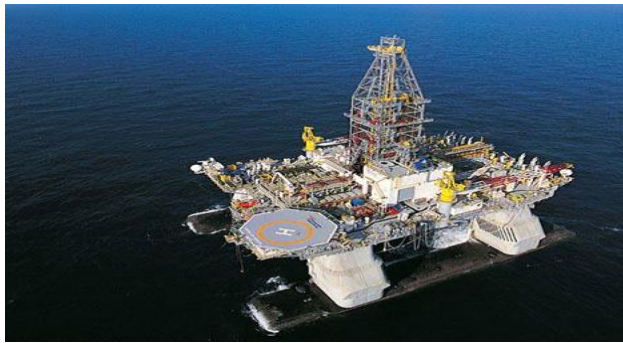
Figure 2. Mobile oil drilling rig positioned on a drilling site.
