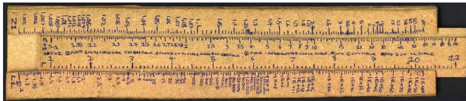
Fig. 1. Slide rule, hand-made made by Robert Munafo at the age of 14.
