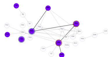
Fig. 2. Argumentation framework: an example of activated arguments (blue nodes inside) given one record of the dataset. Light nodes and edges are still part of the knowledge-base but are not considered for the next layers.
