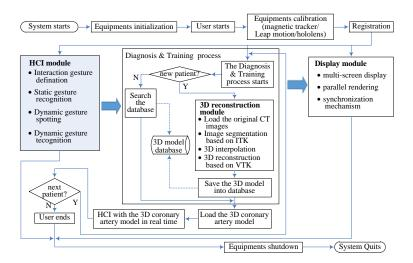
Fig. 2. The workflow and functions of the ARS-CADPT
