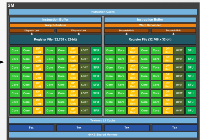
Nvidia Tesla P100 Streaming Multiprocessor (SM) architecture
