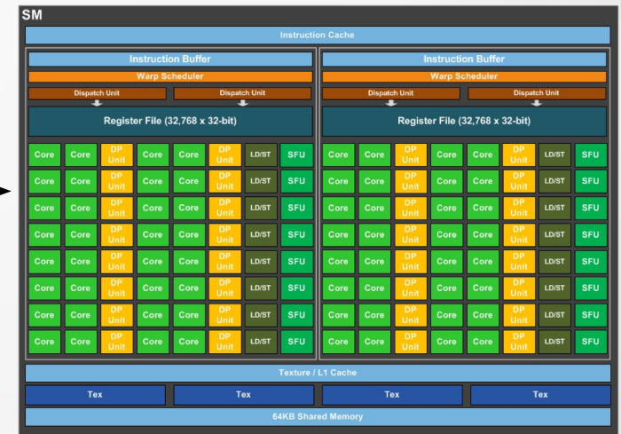
Nvidia Tesla P100 Streaming Multiprocessor (SM) architecture
