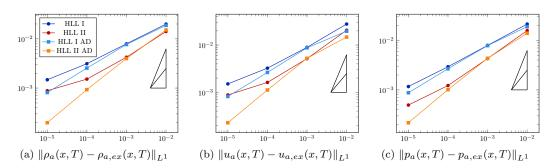
Figure 6: Convergence test for the sensitivity - HLL-type scheme.
