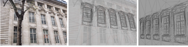
Figure 12: Visualization of the generated facade mesh (center) from the camera of an input view (left). We overlay the input image onto the mesh view to assess alignment. Another viewpoint on the same mesh (right).
