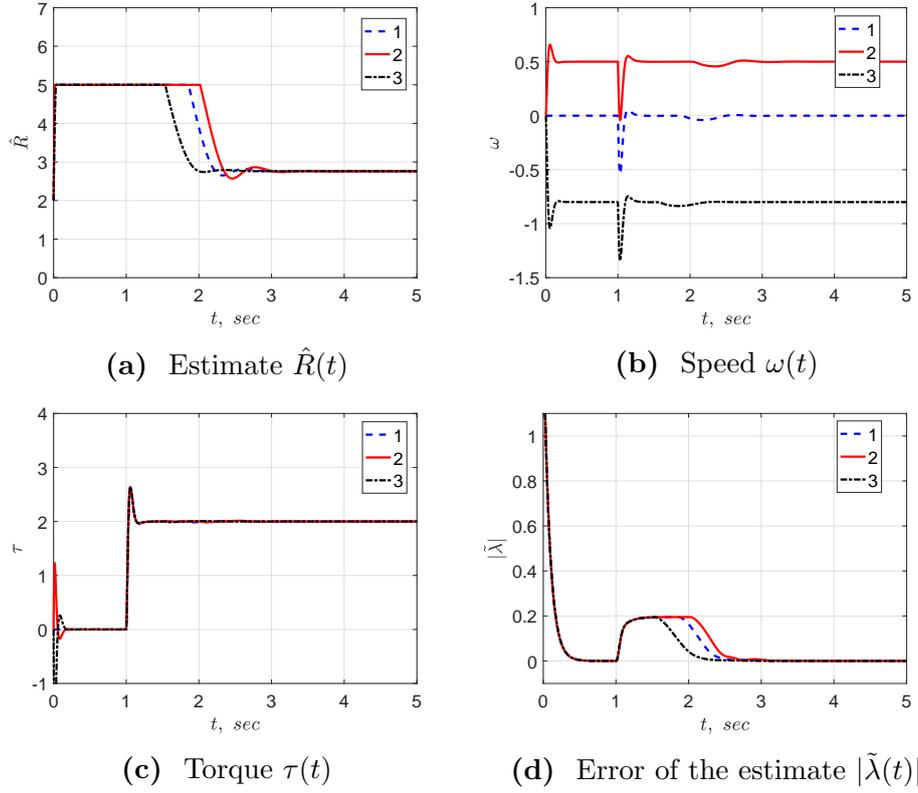
**Figure 8:** Simulation results of the adaptive *speed* regulation IFOC discussed in Section 7 with  $\gamma = 200$ ,  $z(0) = 2$ ,  $\lambda(0) = (0, 0)$ ,  $\hat{\lambda}(0) = (0, 1)$ ,  $a = 50$ , and *different desired speeds*. 1. (blue line)  $\omega_d = 0$ ; 2. (red line)  $\omega_d = 0.5$ ; 3. (black line)  $\omega_d = -0.8$ .
