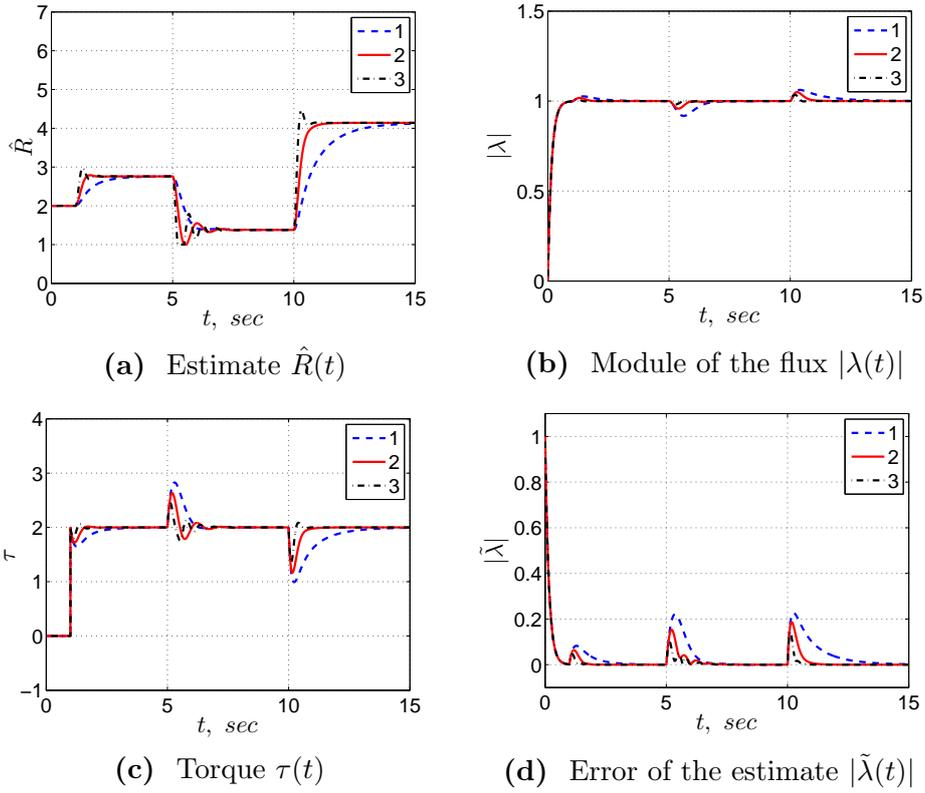
**Figure 4:** Simulation results of the adaptive *torque* regulation IFOC of Proposition 2 with  $z(0) = 2$ ,  $\lambda(0) = (0, 0)$ ,  $\hat{\lambda}(0) = (1, 0)$  *step changes in  $R$  and different adaptation gains.* 1. (blue line)  $\gamma = 30$ ; 2. (red line)  $\gamma = 100$ ; 3. (black line)  $\gamma = 300$ .
