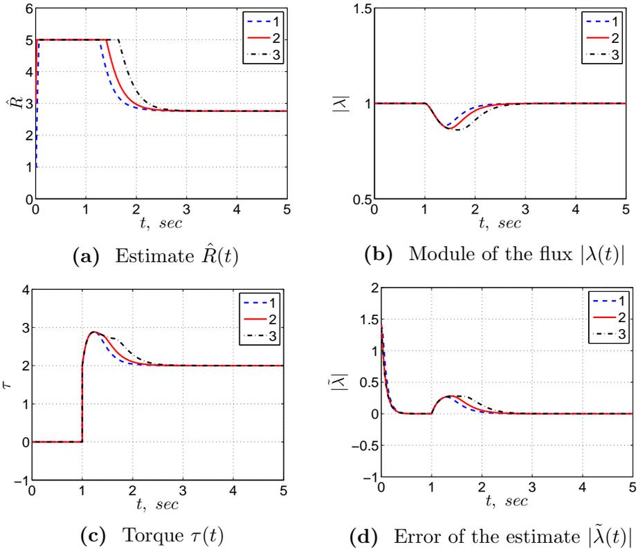
**Figure 2:** Simulation results of the adaptive *torque* regulation IFOC of Proposition 2 with  $\gamma = 100$ ,  $\lambda(0) = (1, 0)$ ,  $\hat{\lambda}(0) = (0, 1)$  and *different initial conditions* for  $z$ . 1. (blue line)  $z(0) = 0$ ; 2. (red line)  $z(0) = 3$ ; 3. (black line)  $z(0) = 5$ .
