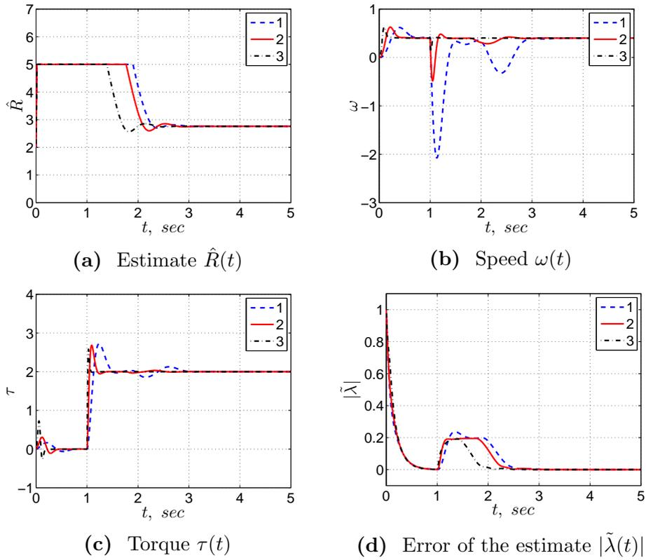
**Figure 7:** Simulation results of the adaptive *speed* regulation IFOC discussed in Section 7 with  $\gamma = 200$ ,  $z(0) = 2$ ,  $\lambda(0) = (0, 0)$ ,  $\hat{\lambda}(0) = (0, 1)$ ,  $\omega_d = 0.4$  and *different values of  $a$* . 1. (blue line)  $a = 10$ ; 2. (red line)  $a = 30$ ; 3. (black line)  $a = 100$ .
