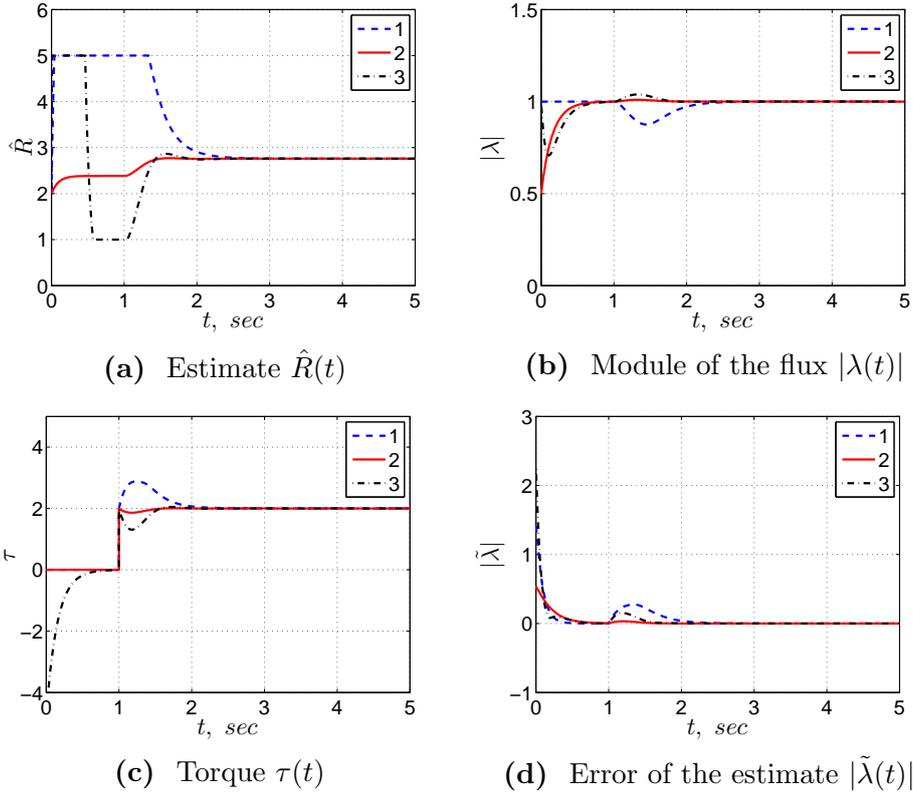
**Figure 3:** Simulation results of the adaptive *torque* regulation IFOC of Proposition 2 with  $\gamma = 100$ ,  $z(0) = 2$  and *different initial conditions for  $\lambda$  and  $\hat{\lambda}$* . 1. (blue line)  $\lambda(0) = (1, 0)$ ,  $\hat{\lambda}(0) = (0, -1)$ ; 2. (red line)  $\lambda(0) = (0.5, 0)$ ,  $\hat{\lambda}(0) = (0, 0.2)$ ; 3. (black line)  $\lambda(0) = (0, 1)$ ,  $\hat{\lambda}(0) = (-1, 3)$ .
