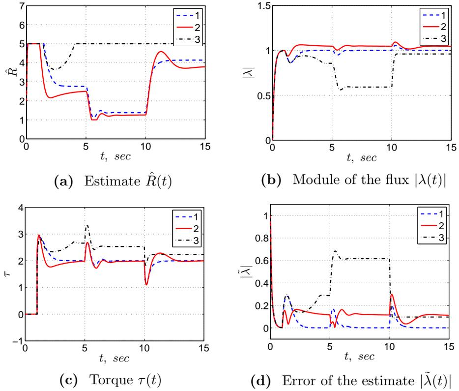
**Figure 5:** Simulation results of the adaptive *torque* regulation IFOC of Proposition 2 with  $\gamma = 50$ ,  $z(0) = 2$ ,  $\lambda(0) = (0, 0)$ ,  $\hat{\lambda}(0) = (0, 1)$  step changes in  $R$  and wrong estimates of  $D$  and  $L$ . 1. (blue line)  $\hat{D} = 0.7D$ ,  $\hat{L} = L$ ; 2. (red line)  $\hat{D} = 0.9D$ ,  $\hat{L} = 1.2L$ ; 3. (black line)  $\hat{D} = 1.2D$ ,  $\hat{L} = 0.95L$ .
