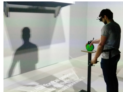
Figure 4: Calibration step – The calibration step enables to compute the offset between the physical ball and the virtual ball at the beginning and end of each virtual shadow condition (N, F or M).
