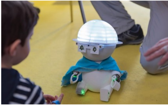
Figure 2: Teegi displays the brain areas involved in vision and motor control of the hands and feet. In order to display these areas, users directly manipulate Teegi's hands and feet, or close his eyes [21].
