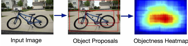
Fig. 3. An illustration of objectness generation process for assessing the easiness of an image sample.
