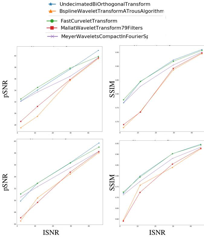
Fig. 3. pSNR (left) and SSIM (right) scores after CS-PI MR image reconstruction from retrospectively under-sampled  $k$ -space data using Sparkling under-sampling schemes (top:  $R = 2.4$ , bottom:  $R = 3.3$ ). Each line codes for a specific multiscale decomposition, see the legend within each panel.
