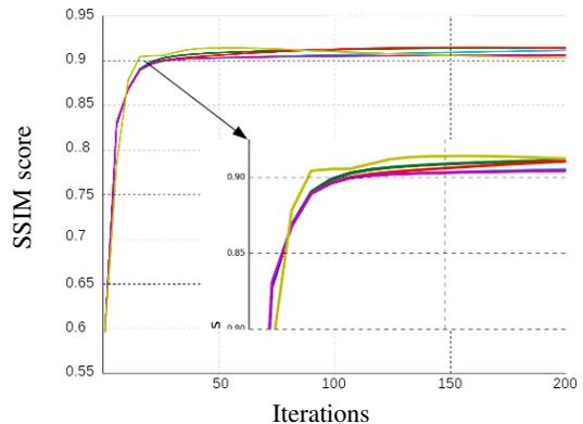
Fig. 2. **Left:** Evolution of the SSIM score over FISTA (yellow curve) and Condat-Vũ (blue, red and green curves) iterations for an orthogonal Mallat WT used as  $\Psi_{\text{OT}}$ . **Insert:** zoom showing that FISTA reaches the SSIM plateau slightly earlier than Condat-Vũ.
