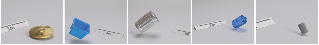
Fig. 12. Falling shells. A set of thin shells are dropped on the ground to produce various nonlinear sounds, including (from left to right) a cymbal, a plastic recycling bin, a galvanized steel trash can, a large plastic bottle, and a small piece of metallic sheet. The one-meter ruler serves as a reference to provide a sense of the physical sizes of the shells. Please refer to the video sound track.
