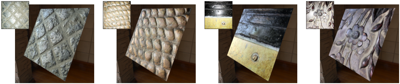
Fig. 1. From a single flash photograph of a material sample (insets), our deep learning approach predicts a spatially-varying BRDF. See supplemental materials for animations with a moving light.
