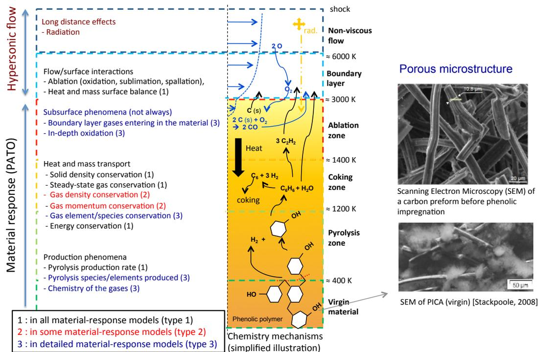
Figure 1: Phenomenology of porous carbon/phenolic ablative materials
