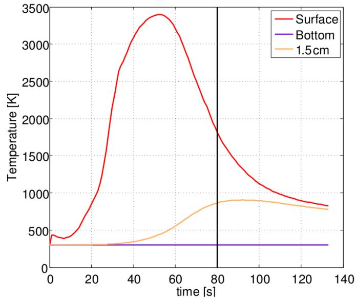
Figure 2: Surface and in-depth temperature obtained with nominal material and pyrolysis gas composition parameters.
