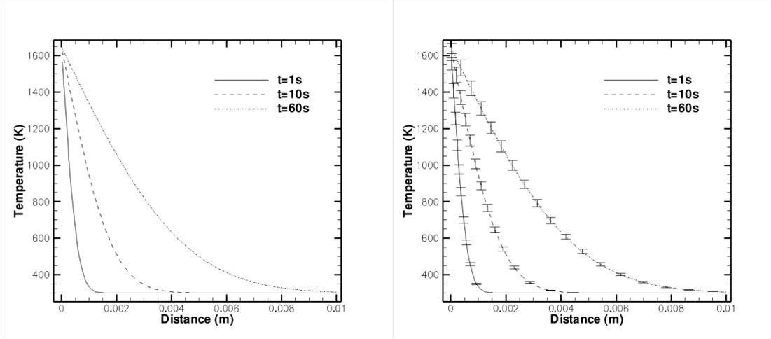
Figure 3: Analytical solution for unidimensional transient heat transfer with fixed surface temperature, for a semi-infinite medium of thermal diffusivity  $10^{-7} m^2/s$ . Initial temperature of the body: 300 K; surface temperature : 1646 K. Left: temperature profiles for 1, 10, and 60 seconds. Right: error bars in terms of standard deviation when considering two uncertainties.
